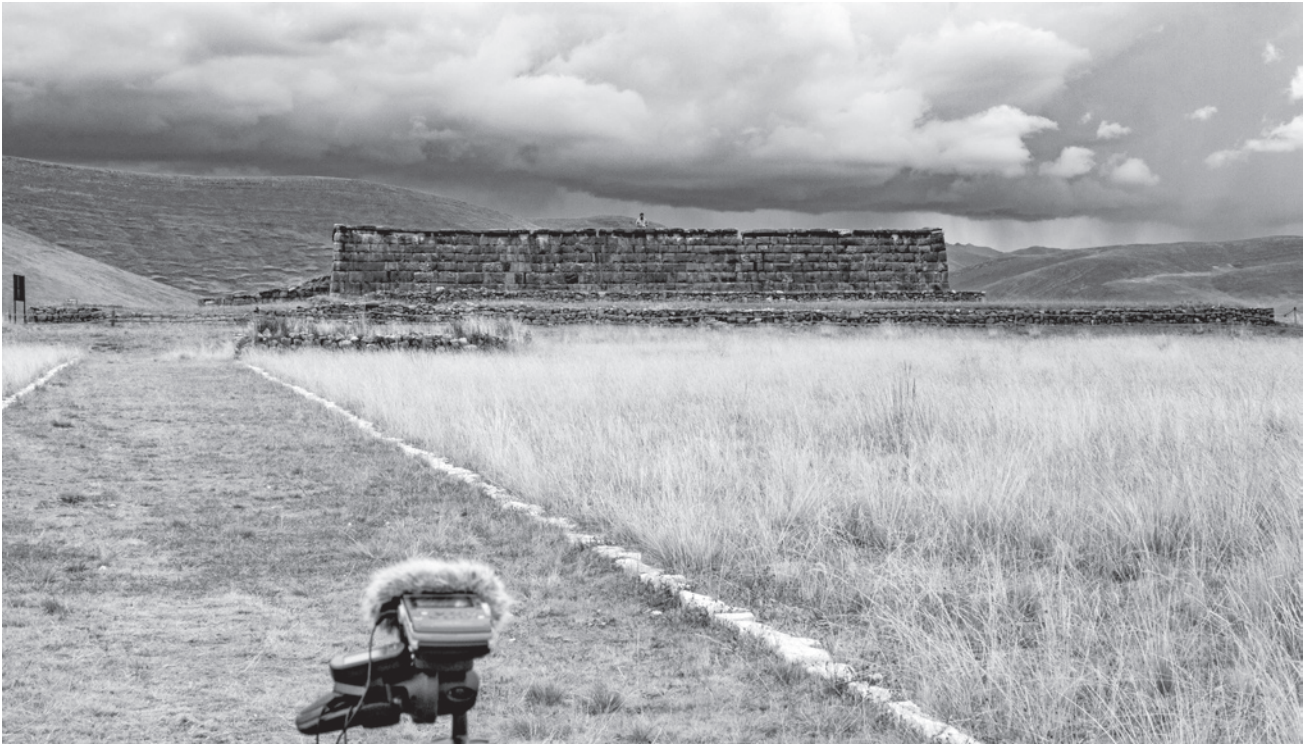
Fig. 1 The central plaza platform (32.5 x 48 m; 4.5 m high) at the Inca administrative center Huánuco Pampa (Peru) served as locus for an experimental acoustical survey of sonic communication and musical instruments conducted in July 2015. In the foreground is the tripod-mounted digital audio recorder with GPS device, approximately 133 m away from the sound-producing performer located centrally at the platform-top's eastern-most wall. Photo (looking west) by Miriam A. Kolar.
